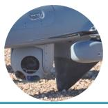
Multi sensors for day and night operations with thermal, infrared and other optics.
